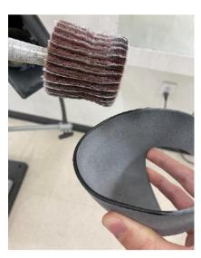
This type of cone does not work as well as it tends to heat and smear the plastic leaving an undesirable finish.
